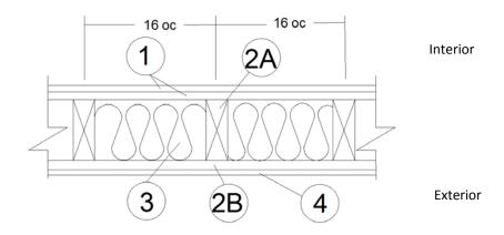
GYPSUM BOARD (Interior): Two layers USG Firecode® C Core, complying with ASTM C1396, or equivalent, min. 5/8 in. thick, 4 ft. wide applied vertically, fastened to framing. Face layer joints staggered with base layer and covered with paper tape and joint compound.
